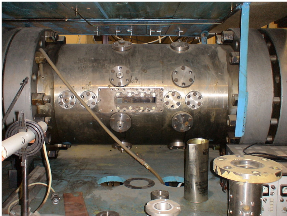
Figure 2.24: Moscow State University Shock Tube
