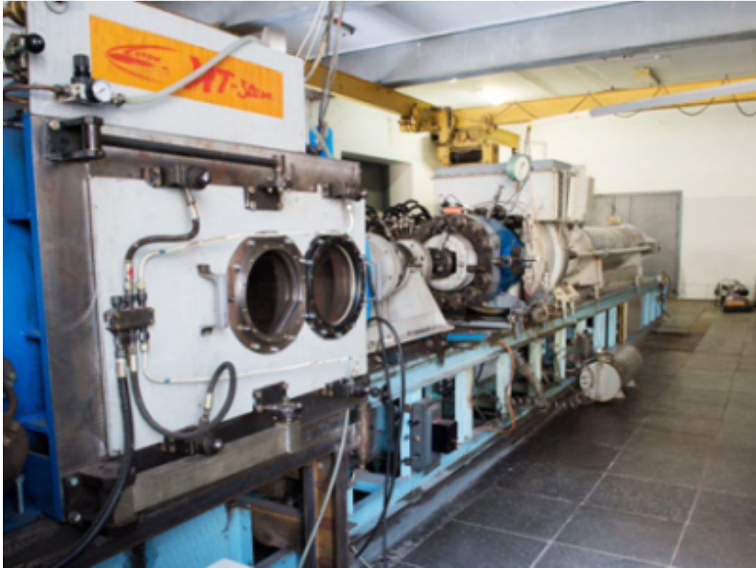
Figure 2.22: ITAM IT-302M hot-shot, adapted from [248]
