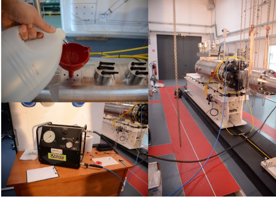
Figure 4.14: Proof-testing with the water pump. Water filling of the combustion chamber and view of the connection to the water pressure pump.
