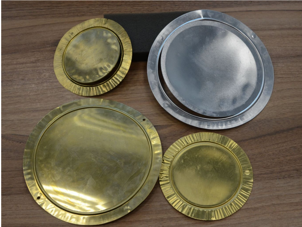
Figure 6.13: Test diaphragms for shock tube section. Tin sheet 0.1 mm (top left) shear cut and buckling; Aluminium sheet 0.3 mm (top right) shear cut; Tin sheet 0.3 mm (bottom left) plastic deformation warped; Tin sheet 0.1 mm (bottom right) plastic deformation buckling.
