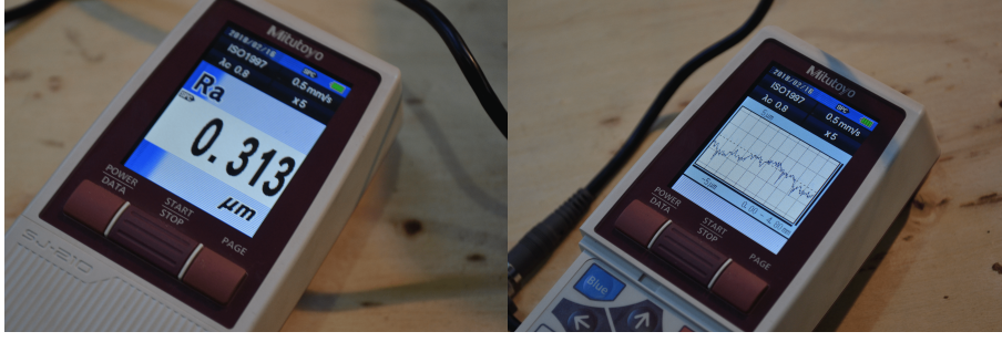
Figure 4.20: Sample surface roughness test using Mitutoyo SurfTest SJ-210.
