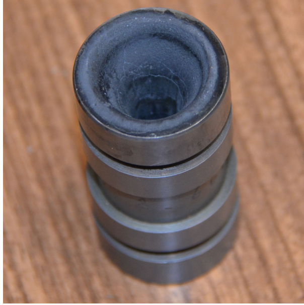
Figure 2.6: ONERA F4 nozzle-throat.
