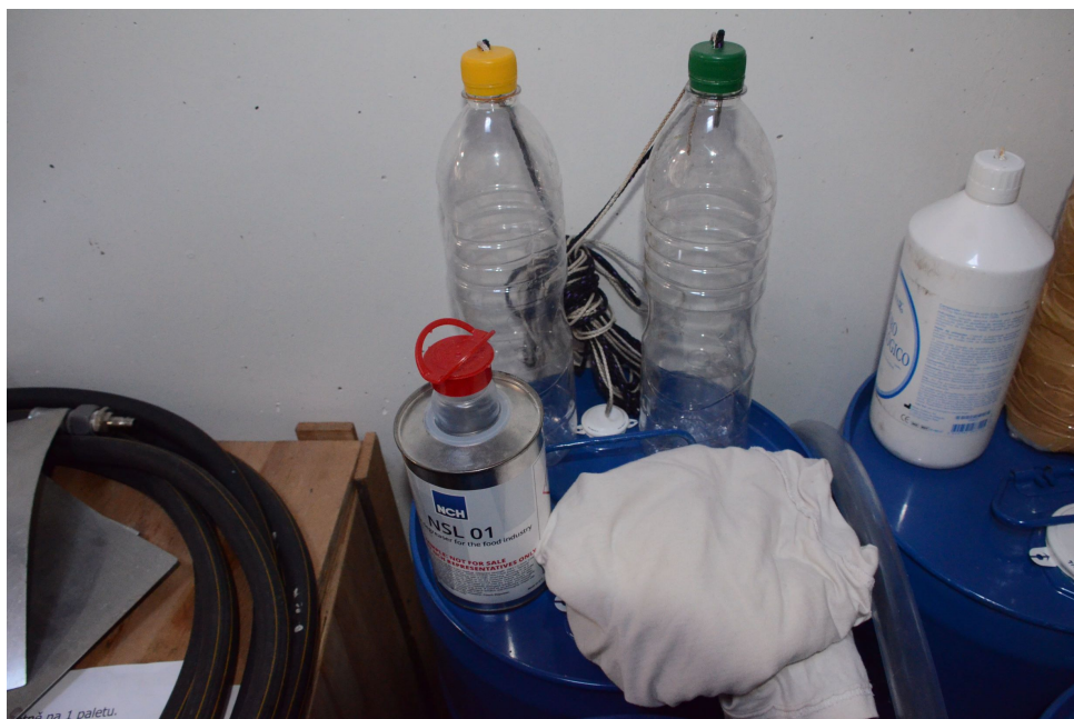
Figure D.2: ESTHER surface cleaning equipment for the shock tube section, two bottles connected by a rope, cotton cloth and cleaning solution. A larger set of bottles is used in the compression tube.
