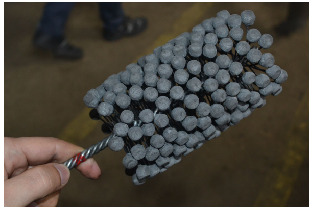
Figure 4.19: FLEX-HONE polishing brush.
