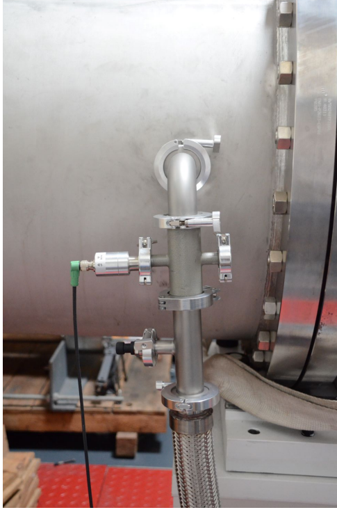
(a) Dump tank, gas port connection and pressure transducers
